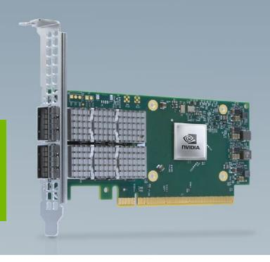
NVIDIA® Mellanox® ConnectX®-6 Dx SmartNIC is the industry's most secure and advanced cloud network interface card to accelerate mission-critical data-center applications, such as security, virtualization, SDN/NFV, big data, machine learning, and storage. The SmartNIC provides up to two ports of 100 Gb/s and one port of 200 Gb/s Ethernet connectivity and delivering the highest return on investment (ROI) of any smart network interface card.
